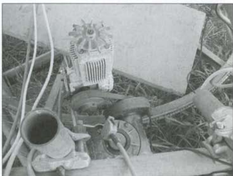
I5PPE + IK5WJD some more details on elevation drive
